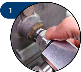
1 Thread coupling fitting into node (due to left-handed threading, coupler will thread simultaneously)
