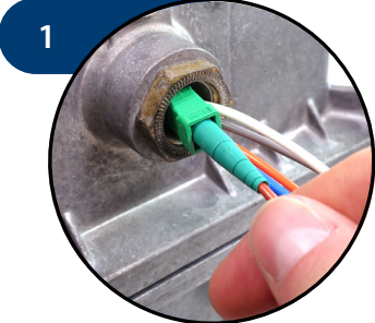
1 Feed connectors through node entry port
