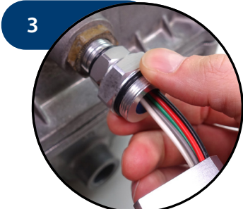
3 Thread coupling fitting a full turn into node
